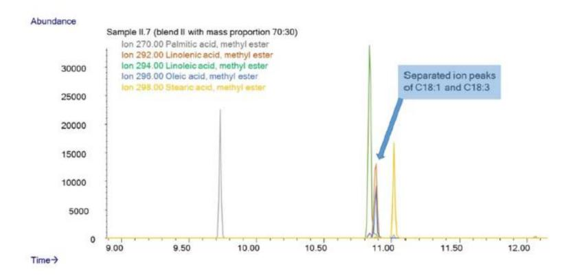
Ion current chromatograms of five prominent FAMEs of sample II.7 showing the extracted ions with the following m/z ratios: 270, 292, 294, 296, and 298.
