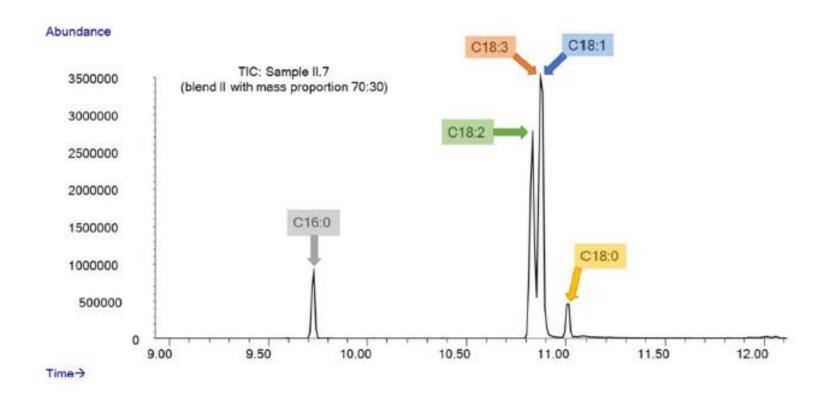
Total ion chomatograms (TIC) obtained by GC-MS of samples: an example of the FO-SO blend.
