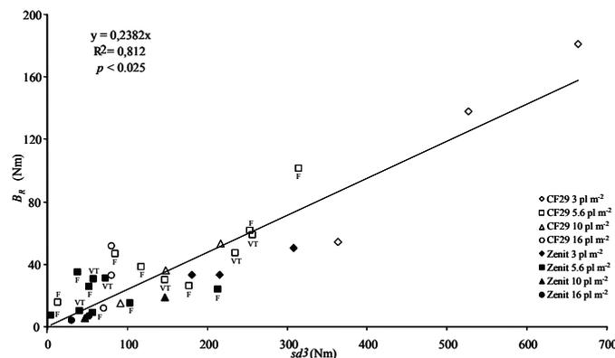
**Fig. 1.** Relation between  $B_R$  (Root failure moment) (Nm) and  $sd^3$  (Plant anchorage) (Nm). Each point is the value for each  $d^3$  (root plate diameter cubed) multiplied by  $s$  (soil shear strength) corresponding to four plant densities (3-5.6-10 and 16 plants  $m^{-2}$ ), two genotypes (Zenit and CF29) and two soil types FAUBA (F), Typic Argiudoll and Venado Tuerto (VT) Typic Hapludoll against each respective value of  $B_R$  (from Sposaro et al., 2008).
